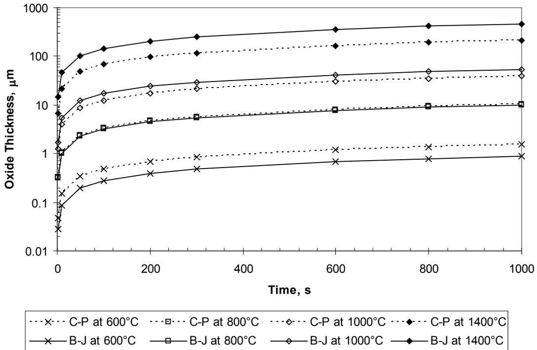
**Figure F.1.** Comparison of C-P and B-J Models at Temperatures from 600 to 1400°C
