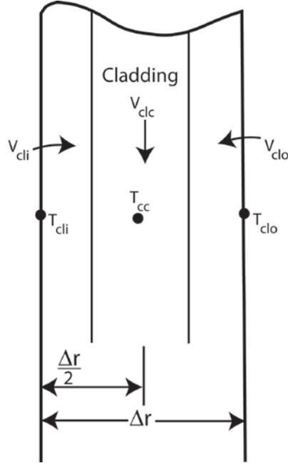
**Figure 2.8.** Cladding Noding
