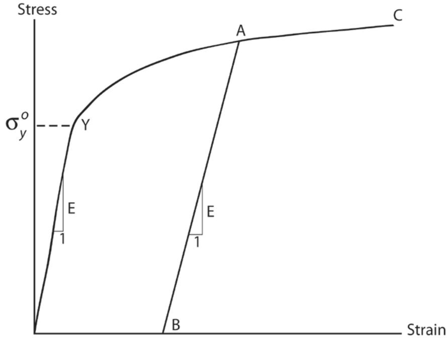
**Figure 2.14.** True Stress-strain Curve and Unloading Path
