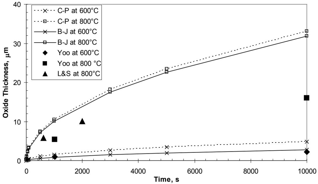
Figure F.2. Comparison of C-P and B-J Models to Data at Temperatures from 600 to 800°C
