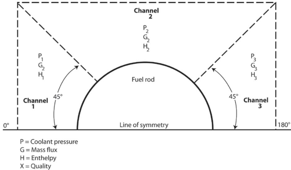
**Figure B.1.** Example Geometry for Input of Coolant Channel Data
