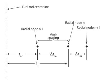
Figure 2.4. Description of Geometry Terms in Finite Difference Equations for Heat Conduction
