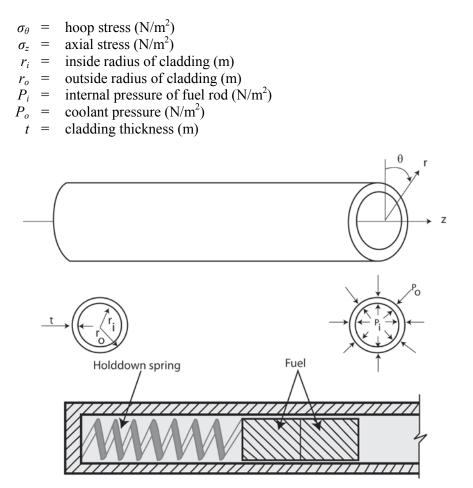
Figure 2.12. Fuel Rod Geometry and Coordinates
