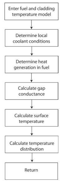
Figure 2.2. Flowchart of Fuel and Cladding Temperature Model (detail of top box of Figure 2.1)
