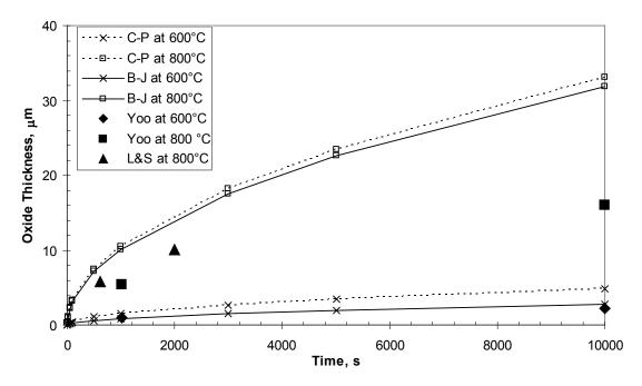
Figure F.2. Comparison of C-P and B-J Models to Data at Temperatures from 600 to 800°C
