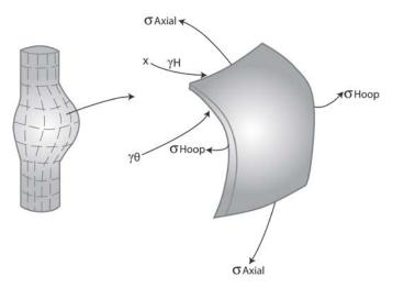
Figure 2.17. Description of the BALON2 Model
