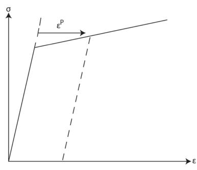
Figure 2.10. Typical Isothermal True Stress-strain Curve
