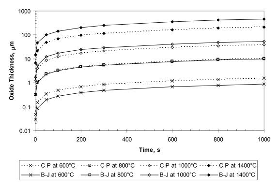
Figure F.1. Comparison of C-P and B-J Models at Temperatures from 600 to 1400°C
