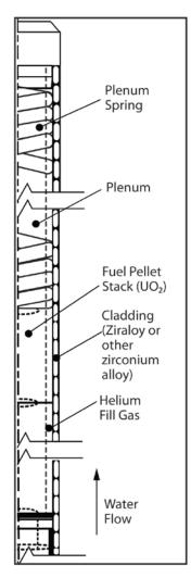
Figure 1.1. Schematic of Typical LWR Fuel Rod
