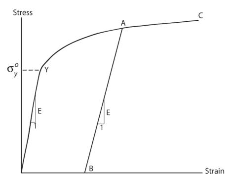
Figure 2.14. True Stress-strain Curve and Unloading Path
