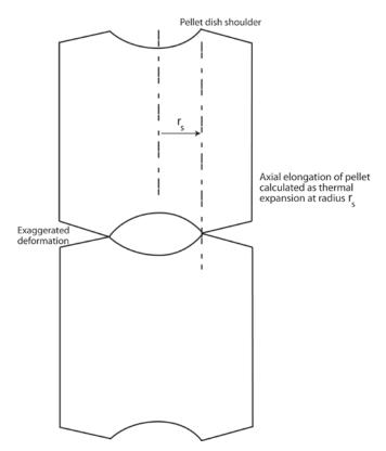
Figure 2.16. Axial Thermal Expansion Using FRACAS-I
