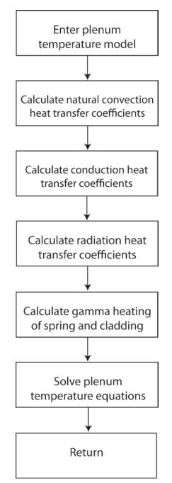
Figure 2.7. Flowchart of Plenum Temperature Calculation
