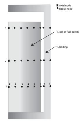
Figure 3.4. Example of Fuel Rod Nodalization
