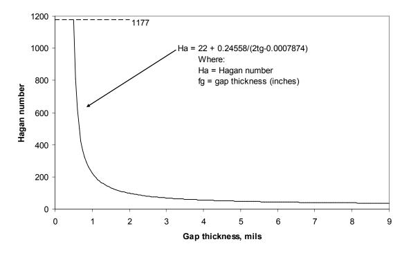
Figure 2.24. Hagen Number Versus Width of Fuel-Cladding Gap
