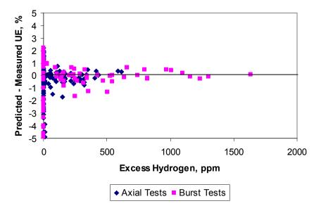
**Table 2.5**.Predicted Minus Measured Uniform Elongation from Irradiated Samples from the PNNL<br/>Database as a Function of Excess Hydrogen ( $293K \le T \le 755K$  and  $0 \le \Phi \le 14 \times 10^{25}$  n/m<sup>2</sup>)
